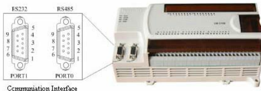
Figure 2-7-4 LM3108 Communication Interface
